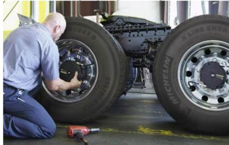
Two years ago, a California startup named <u>Aperia Technologies</u> began selling a solution to this problem: the hub-mounted Halo Tire Inflator. Similar to a self-winding watch, it uses a pendulum-type weight to power a pump as the wheel it's attached to turns. Set to a specific pressure, the device is connected to the tire's valve stem via a hose and automatically increases or reduces pressure as needed. One Halo can serve up to two tires.
