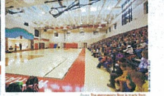
Photo: The gymnasium floor is made from sustainable bamboo. The joists from the old gymnasium was recycled for the building's structure. Classroom windows are made from recycled glass.
