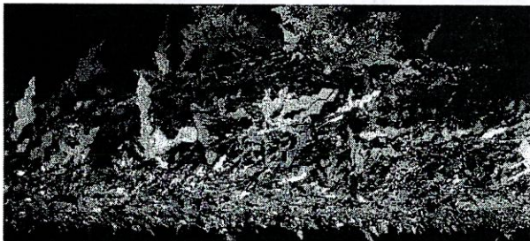
Uranium dendrites collected during the evaluation of Argonne's advanced electrorefining technology.
