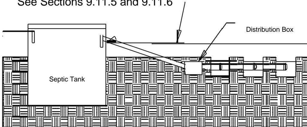
Note: Capping material must extend 10 ft. from trenches before the start of the slope. The tapered slope shall be 3:1 or less.
