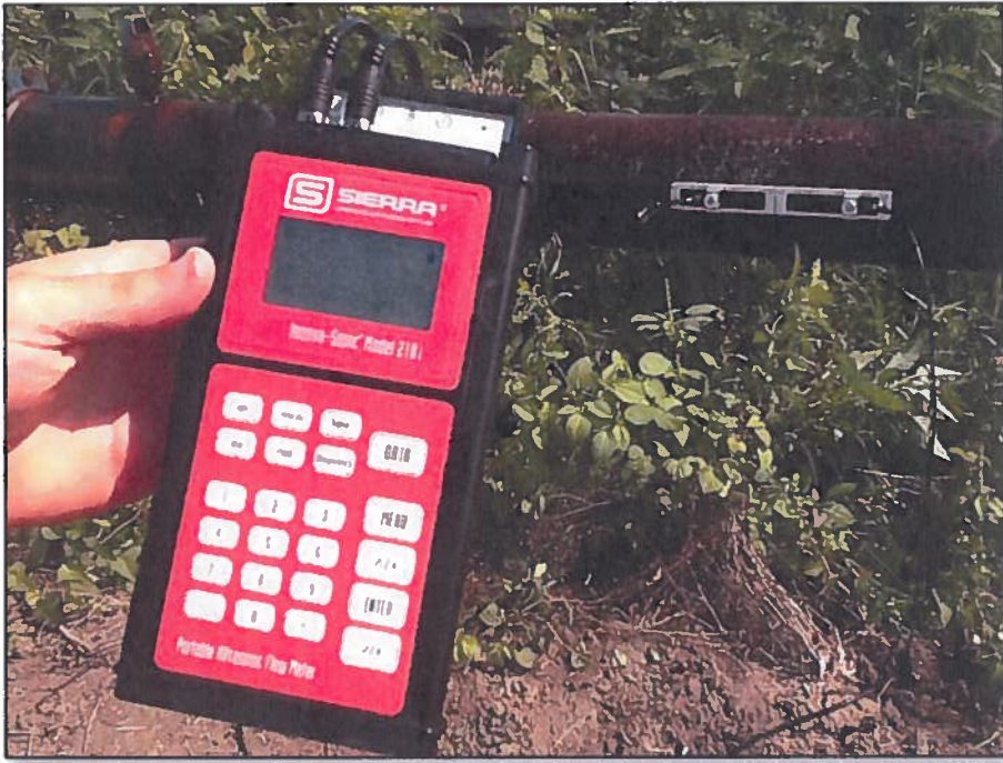
Flow rate measurement for calibrating pumps to increase efficiency
