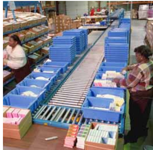
Figure 3-118: Flow Racks in South Carolina Warehouse
