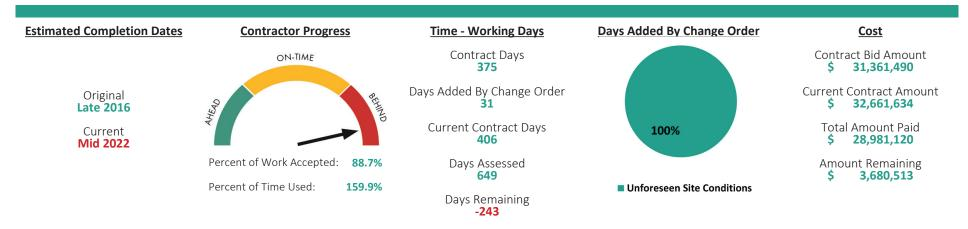
This project has experienced delays due to adverse weather and production issues. The cost has increased due to additional piling required for footing construction. Additional delays have been experienced due to girder displacement following concrete deck placement. Utility conflicts have also caused delays with paving on the south end of the project.
