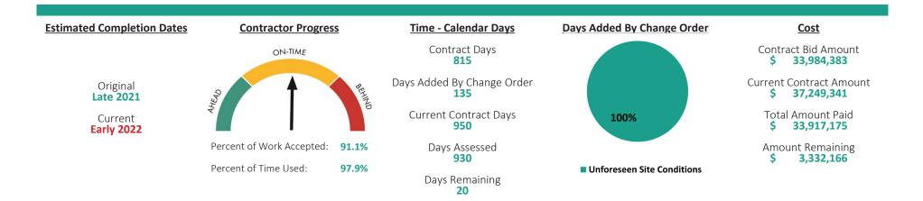
The cost for this project has increased approximately \$3.4 million which is primarily due to slide repairs at various locations throughout the project that occurred after being let to contract. The contract time has been increased by 135 calendar days for the slide repair work.
