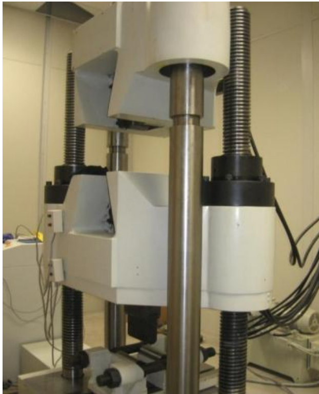
Universal Testing Machine 200,000 lb load capacity
