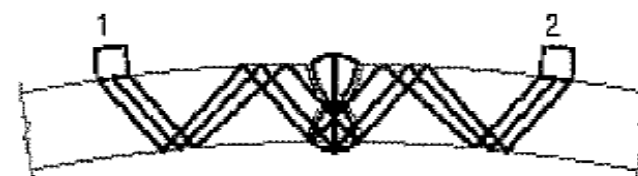
PROBE PAIR FOR INNER ZONE (LONGITUDINAL DEFECT)
