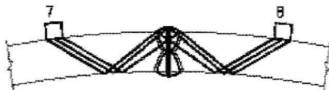
PROBE PAIR FOR OUTER ZONE (LONGITUDINAL DEFECT)
