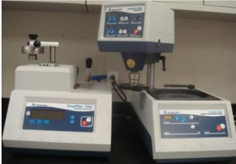
Sample Mounting & Automatic Polishing Machine
