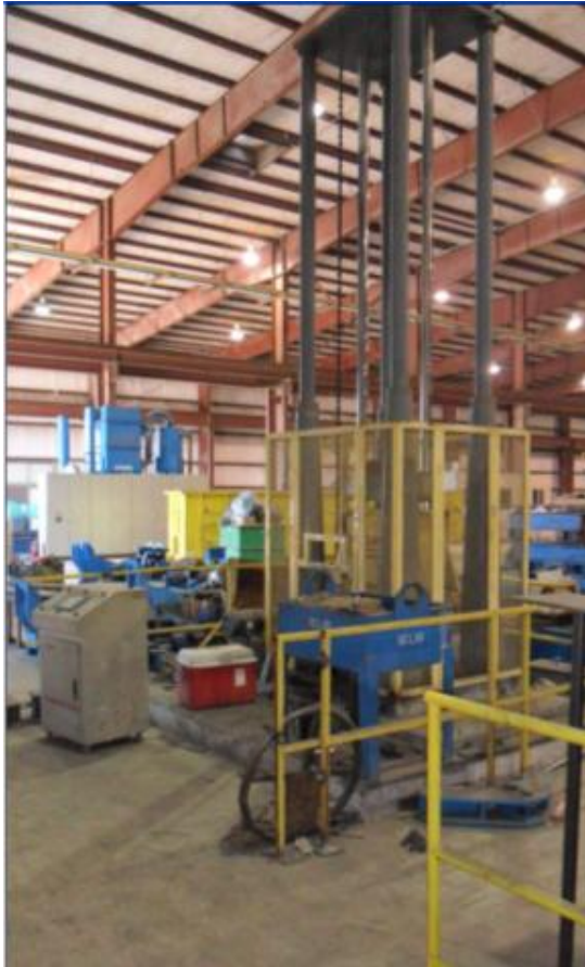
Drop Weight Impact Testing Machine 22,000 ft-lb capacity
