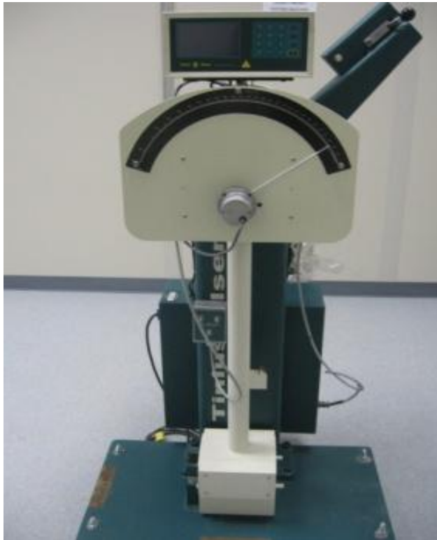
Charpy Impact Testing Machine 330 ft-lb capacity
