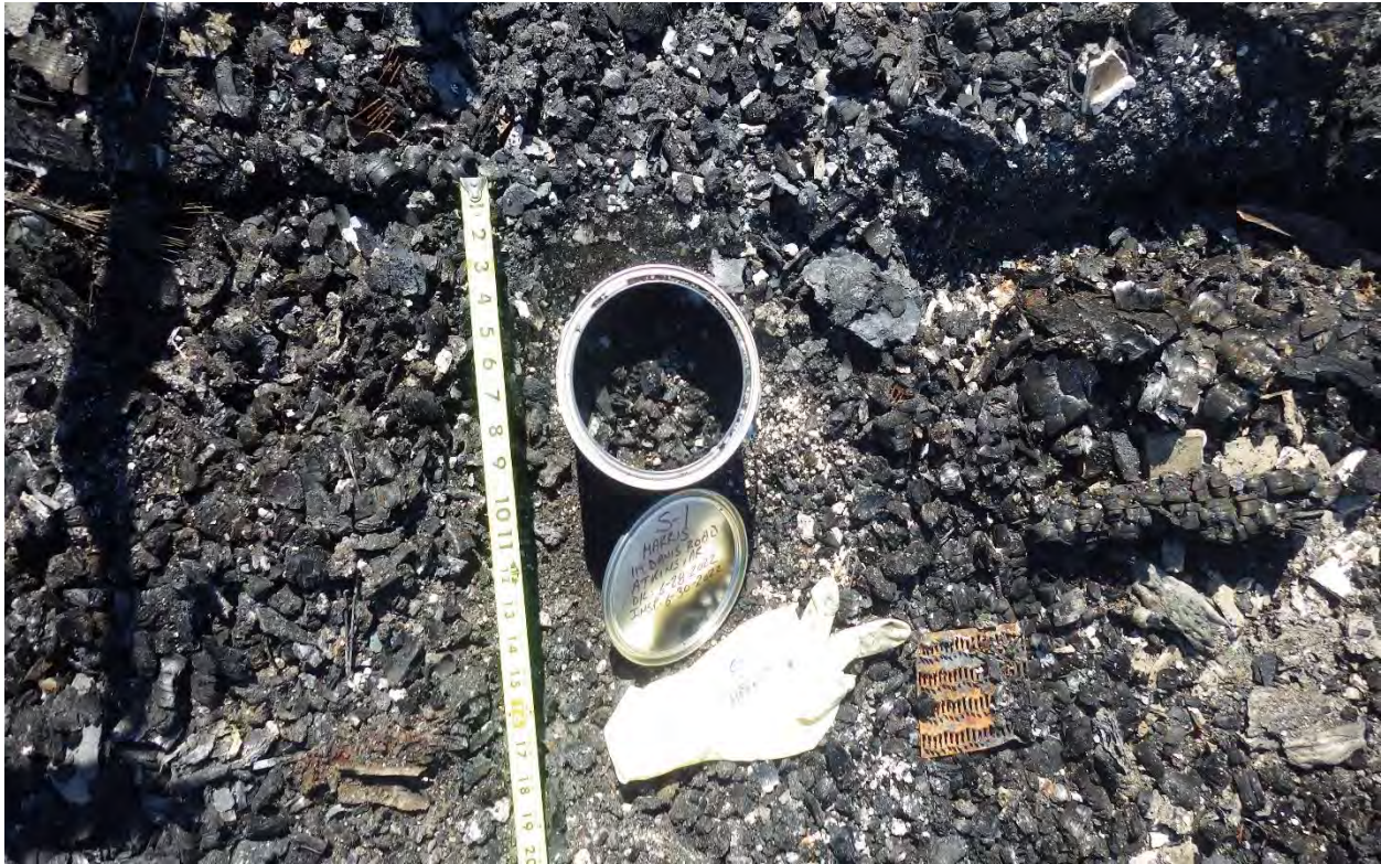
Photo No. 21: View of debris sample S-1 collected from area of fire origin
