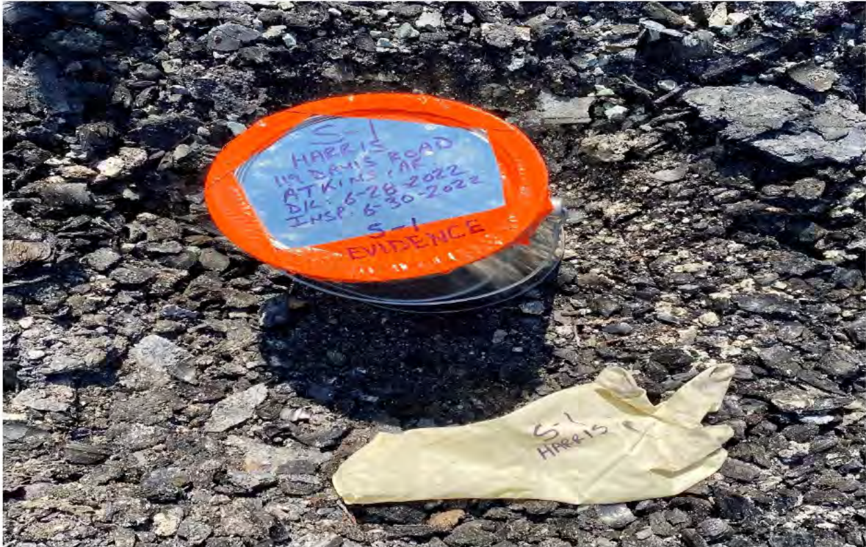
Photo No. 23: View of sealed sample S-1 collected at ground level below front door entrance
