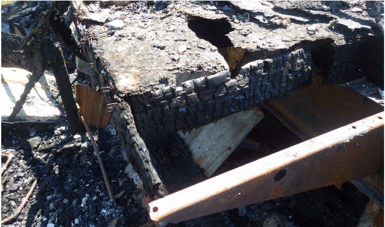
Photo No. 19: View of loss of mass, directional, tempering and depth of char fire patterns
