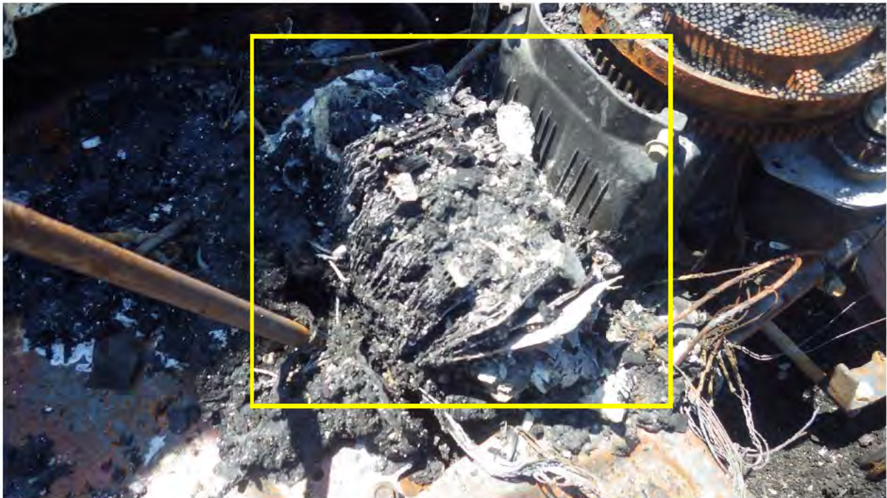
Photo No. 16: View of remains of battery on riding mower
