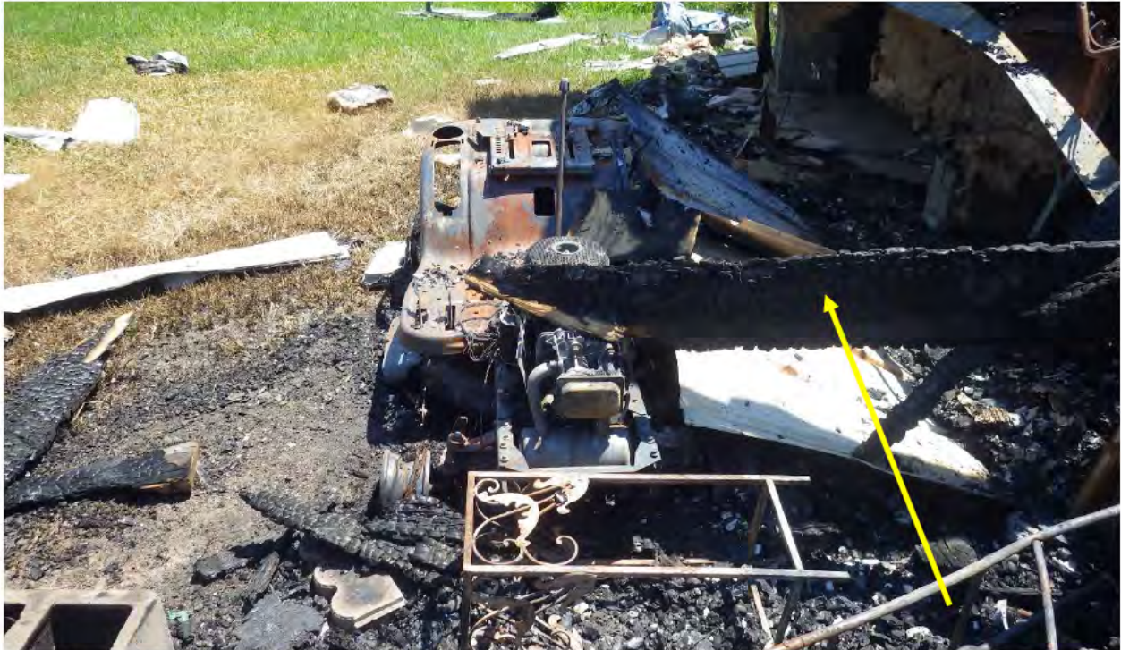
Photo No. 15: View of riding lawn mower parked at south end of wood deck, note fire patterns on inside of wood deck framing (shown with yellow arrow)
