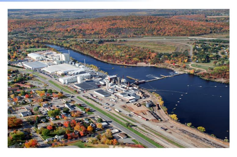
Today the mill operates one pulp line and one paper machine with a production capacity of 147,000 Tons per year.
